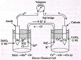
The deflection in voltmeter indicates that there is a potential difference between the two electrodes. It has been found that the conventional current flows through the outer circuit from copper to zinc strip. It implies that the electrons flow occures from zinc to copper strip.
