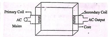
The efficiency of transformer—Efficiency of transformer is defined as, It is ratio of output power to the input power.
