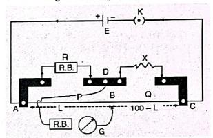
The connections are made as shown in figure. A resistance R is introduced from the resistance box and the key K is closed. The jockey is moved on the wire to the point where there is no deflection in the galvanometer. In such a case points B and D are at the same potential. The point B is called the 'null' point.
